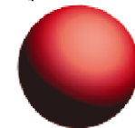
Dia. 0,5mm Uranium Dioxide Fuel Kernel
